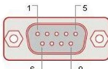
A diagram of a DB9 male connector showing its pin layout. It has two metal nuts at the ends. There are 9 pins in total, arranged in three rows of three. Pin 1 is at the top left, Pin 5 is at the top right, Pin 6 is at the bottom left, and Pin 9 is at the bottom right. |
